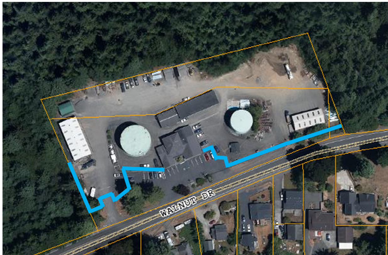
Figure 2: Diagram showing the extents of the fence to be rehabilitated in blue.
